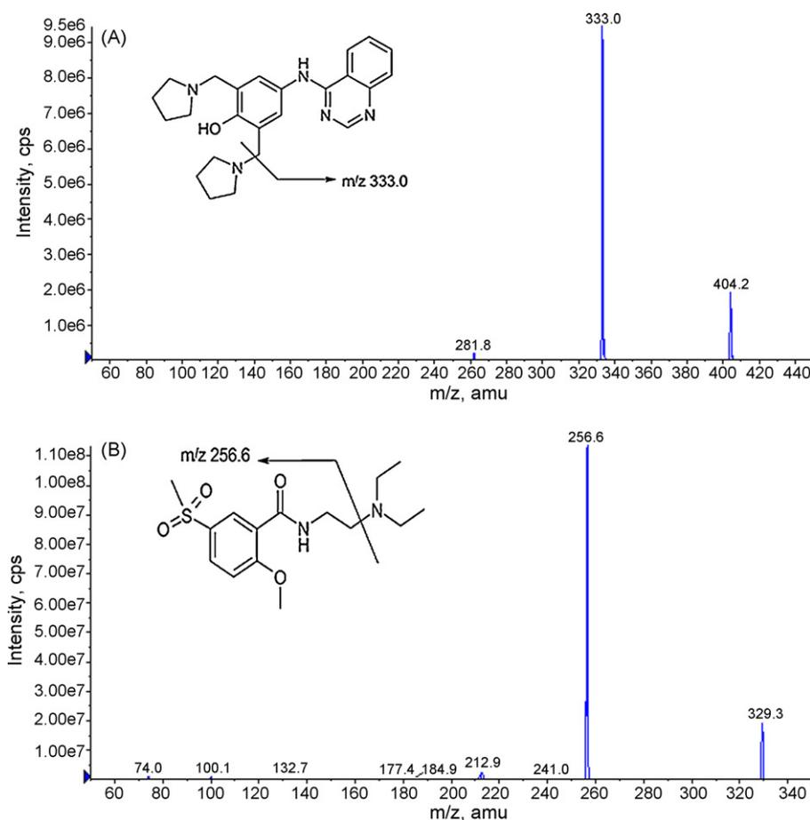
Fig. 1. Product ion mass spectra of changrolin (A) and internal standard tiapride (B).
